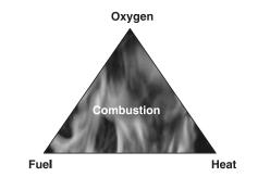
Figure 8.1 The fire triangle. A fire needs three things to survive: heat, oxygen, and fuel. A fire may be effectively suppressed by removing any of these elements.
