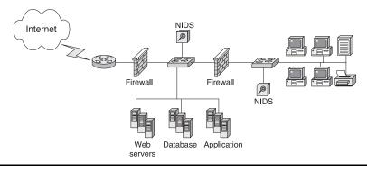
Figure 7.3 NIDS deployment. A network-based intrusion detection system (NIDS) analyzes network traffic. NIDS are deployed as network devices running in promiscuous mode.
