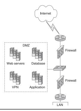
Figure 7.1 A demilitarized zone (DMZ) is a secure network architecture configuration in which publicly accessible services are separated from the rest of the network by employing firewall technology.
