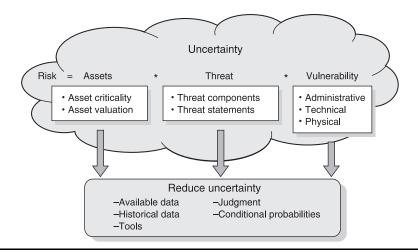
Figure 9.2 Introduction of uncertainty into determining risk. The basic components of the risk equation are clouded by uncertainty. Uncertainty may be reduced by gathering additional information or using consensus techniques.
