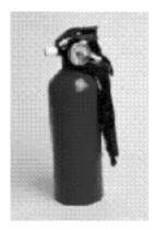
Figure 8.4 Mobile suppression systems. Commonly referred to as handheld fire extinguishers, these devices should be placed within 50 feet of equipment toward the door, inspected monthly, and tested annually.
