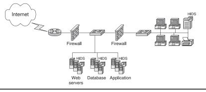
Figure 7.2 HIDS deployment. A host-based intrusion detection system (HIDS) inspects packets sent to the host. HIDS are deployed as software agents running on the host.
