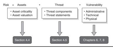
Figure 9.1 Basic risk equation. The basic risk equation computes the relationship between assets, threats, and vulnerabilities. Each of these areas has been covered in a previous section of this book.
