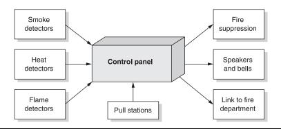
Figure 8.3 Fire alarm systems. A fire alarm system is an interconnected protection system consisting of fire detectors, pull stations, fire suppression equipment, speakers, a control panel, and optionally a link to the fire department.
